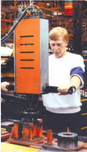
Repair bay operator is using a two spindle fixtured tool to fasten components of a wheel hub assembly.
